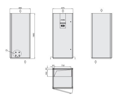
1 Pipe connect area: Specific position and kinds differ slightly in different unit series. Refer to the onsite unit.
