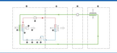
1 Indoor unit 2 Outdoor unit 3 Pump group(optional) 4 Dry cooler(optional) 5 Compressor 6 Evaporator 7 Supply fan
