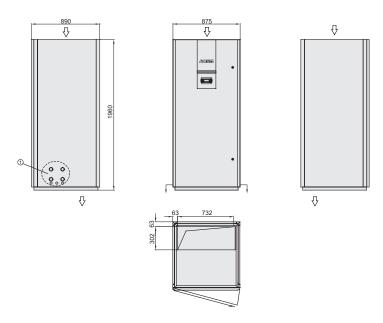
① Pipe connect area: Specific position and kinds differ slightly in different unit series. Refer to the onsite unit.
